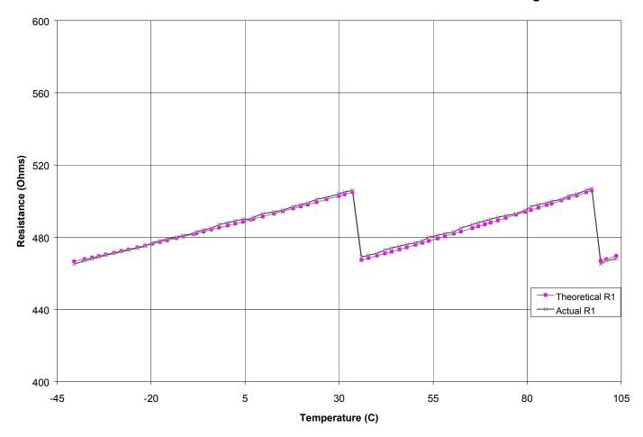
The results of the experiment indicate the equation very accurately calculates the value of the resistance for low-position settings. The accuracy in this particular case was always within  $\sim\!2\Omega$  of the expected value. Also note that even with compensation the resistance changes over temperature. It can only be compensated to within 1/2LSB best case, and thus the designer must allow for the some quantization error when designing the system.
