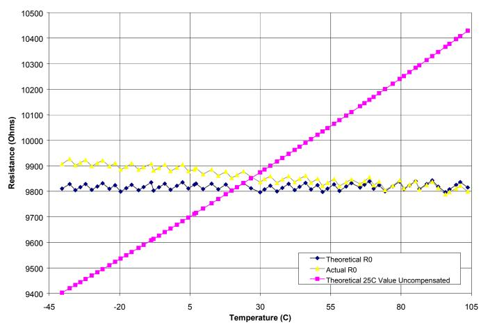
Resistor 0's LUT was loaded with values corresponding to approximately the maximum resistance that can be maintained over temperature. The maximum resistance for this part was approximately  $9820\Omega$ . The experiment was repeated, and the results were again plotted. This time an additional function was added that shows how the uncompensated room temperature resistance (a theoretical value, no lab data was acquired) would fair over temperature as well.
